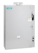
Pump control panel, Size 4, Three phase full voltage, Solid-state overload relay, OLR amp range 50-200A, 110V 50Hz / 120V 60Hz coil, Standard type contactor, 200A fusible disconnect, 200A/600V fuse clip, HOA Sel Sw. <(>&<)> Start P.B., Enclosure NEMA type 3/3R, Weather proof outdoor use
