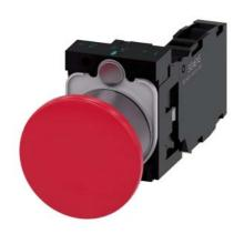
Mushroom pushbutton, 22 mm, round, plastic with metal front ring, red, 40 mm, latching, pull-to-unlatch mechanism, with holder, 1 NO+1 NC, screw terminal
