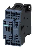
Power contactor, AC-3 38 A, 18.5 kW / 400 V 1 NO + 1 NC, 24 V DC 3-pole, size S0 Spring-type terminals
