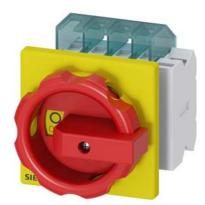
SENTRON, Switch disconnector 3LD, emergency switching-off switch, 3-pole, Iu: 16 A, operating power / at AC-23 A 400 V: 7.5 kW, front-mounted, 1 NC, 1 NO, rotary operating mechanism, Red / yellow, 4-hole mounting of the handle
