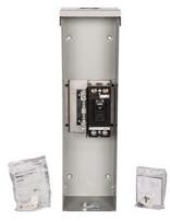
SIEMENS LOW VOLTAGE POWER MOD WB STANDARD CIRCUIT BREAKER MAIN. 1-PHASE 3-WIRE SYSTEM RATED 120/240V (800A) 65KAIC INTERRUPT. SPECIAL FEATURES: NEMA TYPE 3R ENCLOSURE, OH/UG SERVICE FEED. 800A 2-POLE MXD6 FRAME BREAKER INCLUDED (MXD62B800). FACTORY INSTALLED LUGS.
