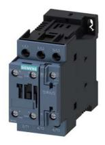
Power contactor, AC-3 38 A, 18.5 kW / 400 V 1 NO + 1 NC AC (50 - 60 Hz) / DC 200-280 V AC / DC, 3-pole Size S0, screw terminals Size S0, screw terminals
