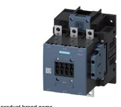
Power contactor, AC-3 150 A, 75 kW / 400 V AC (50-60 Hz) / DC operation 110-127 V UC Auxiliary contacts 2 NO + 2 NC 3-pole, Size S6 Busbar connections Drive: conventional screw terminal
