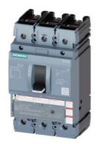
circuit breaker 3VA5 UL frame 250 breaking capacity class H 65kA @ 480 V 3-pole, line protection TM210, FTFM, In=200A overload protection Ir=200A fixed short-circuit protection li=10 x In cable connection on both sides
