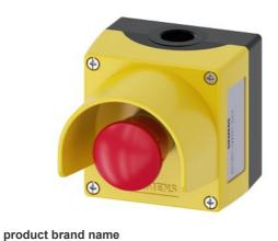
Enclosure for command devices, 22 mm, round, Enclosure material metal, Enclosure top part yellow, with protective collar, 1 control point metal, A=EMERGENCY STOP mushroom pushbutton red, 40 mm, rotate-to-unlatch, 1 NO, 1 NC, 1 NC, screw terminal, floor mounting, 1xM20 each on top and bottom
