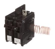
Siemens Low Voltage Molded Case Circuit Breakers General Purpose MCCBs are Circuit Protection Molded Case Circuit Breakers. 1-Pole circuit breaker type BQ. Rated 120V (020A) (AIR 10 kA). Special features: 120VAC Shunt Trip. Note: Load side lugs are included.
