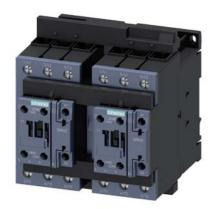
Reversing contactor assembly AC-3, 37 kW/400 V 110 V AC 50 Hz/120 V 60 Hz, 3-pole Size S2, screw terminal electrical and mechanical Interlock 2 NO integrated
