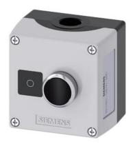
Enclosure for command devices, 22 mm, round, Enclosure material metal, enclosure top part gray, 1 control point metal, A=Pushbutton black, 1 NC, screw terminal, floor mounting, label: O, 1xM20 each on top and bottom, Label enclosed
