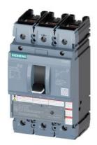
circuit breaker 3VA5 UL frame 250 breaking capacity class M 35kA @ 480 V 3-pole, line protection TM210, FTFM, In=175A overload protection Ir=175A fixed short-circuit protection Ii=10 x In cable connection on both sides
