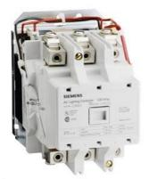
Mechanically held lighting contactor, Contactor amp rating 100A, 0 N.C. / 3 N.O. poles, 220VAC 50HZ/240VAC 60HZ coil, Non-combination type, Enclosure NEMA type (open), No enclosure
