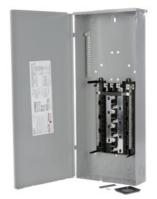
SIEMENS LOW VOLTAGE PL SERIES LOAD CENTER. MAIN LUG WITH 24 1-INCH SPACES ALLOWING MAX 42 CIRCUITS. 3-PHASE 4-WIRE SYSTEM RATED 120/240V OR 120/208V (200A) 100KA INTERRUPT. SPECIAL FEATURES: COPPER BUS, INTERCHANGEABLE MAIN, GRAY TRIM, NEMA TYPE3R ENCLOSURE FOR OUTDOOR USE.
