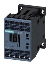
Power contactor, AC-3 7 A, 3 kW / 400 V 1 NO, 110 V AC, 50 Hz 120 V, 60 Hz, 3-pole, Size S00, Spring-type terminal
