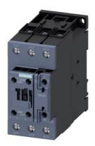
Power contactor, AC-3 65 A, 30 kW / 400 V 1 NO + 1 NC, 175-280 V AC/DC with varistor 3-pole, size S2 screw terminals
