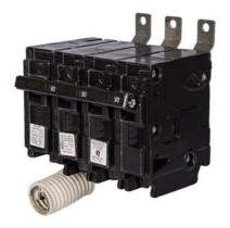
Siemens Low Voltage Molded Case Circuit Breakers Panelboard Mounting 240V Circuit Breakers - Type BL, 3-Pole, 240VAC are Circuit Protection Molded Case Circuit Breakers. Type: BLH Special Features: Shunt Trip 120V Application: Electrical Distribution Standard: UL 489 Voltage Rating: 120/240V Amperage Rating: 20A Trip Range: Thermal Magnetic Interrupt Rating: 22 AIC Number Of Poles: 3P
