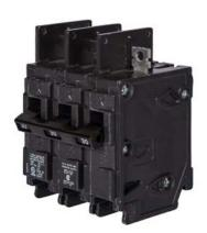
Siemens Low Voltage Molded Case Circuit Breakers General Purpose MCCBs are Circuit Protection Molded Case Circuit Breakers. 3-Pole Common-Trip circuit breaker type BQ. Rated 240 V (025A) (AIR 10 kA). Special features: Load side lugs are included.
