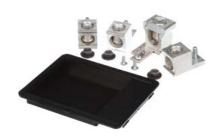
Aluminum (Main or Feed-Thru) Lug kit for original P1 interior panelboard. Suitable for 3-Phase system rated (250A). Wire range: No.6 AWG - 350kcmil (CU/AL). Not suitable for use with Revised P1 panels produced after December 2014.
