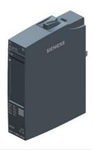
SIMATIC ET 200SP, Digital input module, DI 8x 24V DC SRC BA, type 1 (IEC 61131), source Input (NPN, M-reading) Packing unit: 1 piece, fits to BU-type A0, Colour Code CC02, input delay time 0,05..20ms, module diagnostics for: supply voltage
