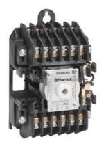
Mechanically held lighting contactor, Contactor amp rating 20A, 0 N.C. / 3 N.O. poles, Non-combination type, Enclosure NEMA type (open), No enclosure
