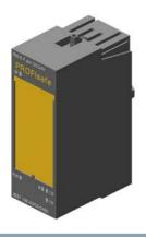
SIMATIC DP, Power Module PM-E F PROFIsafe, f. ET200S; 24 V DC suitable for ungrounded setup relay for switching the voltage buses P1 and P2 up to Category 3 (EN 954-1)/ SIL2 (IEC61508)/PLD (ISO13849), 2 fail-safe dig. outputs up to Category 4 (EN 954-1)/ SIL3 (IEC61508)/PLE (ISO13849), can also be used in PROFINET configuration with IM 151-3 HF
