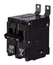
Siemens Low Voltage Molded Case Circuit Breakers Panelboard Mounting 240V Circuit Breakers - Type BL, 2-Pole, 120/240VAC are Circuit Protection Molded Case Circuit Breakers. Type: BL Application: Electrical Distribution Standard: UL 489 Voltage Rating: 120/240V Amperage Rating: 45A Trip Range: Thermal Magnetic Interrupt Rating: 10 AIC Number Of Poles: 2P
