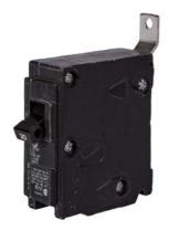
Siemens Low Voltage Molded Case Circuit Breakers Panelboard Mounting 240V Circuit Breakers - Type BL, 1-Pole, 120VAC are Circuit Protection Molded Case Circuit Breakers. Type: BLH Application: Electrical Distribution Standard: UL 489 Voltage Rating: 120V Amperage Rating: 45A Trip Range: Thermal Magnetic Interrupt Rating: 22 AIC Number Of Poles: 1P
