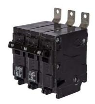
Siemens Low Voltage Molded Case Circuit Breakers Panelboard Mounting 240V Circuit Breakers - Type BL, 3-Pole, 240VAC are Circuit Protection Molded Case Circuit Breakers. Type: BL Application: Electrical Distribution Standard: UL 489 Voltage Rating: 240V Amperage Rating: 90A Trip Range: Thermal Magnetic Interrupt Rating: 10 AIC Number Of Poles: 3P
