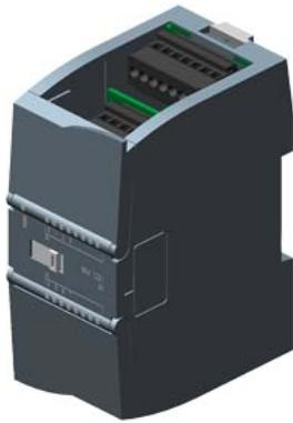
SIMATIC S7-1200, Analog input, SM 1231, 8 AI, +/-10 V, +/-5 V, +/-2.5 V, or 0-20 mA/4-20 mA, 12 bit+sign or (13 bit ADC)
