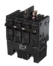
Siemens Low Voltage Residential Circuit Breakers Main Breakers - Type QPP/MPP Breakers are Circuit Protection Load Center Mains, Feeders, and Miniature Circuit Breakers. Type: QPPH Application: Electrical Distribution Standard: UL 489 Voltage Rating: 120/240 V Amperage Rating: 200A Trip Range: Thermal Magnetic Interrupt Rating: 22 AIC Number Of Poles: 2P
