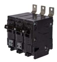
Siemens Low Voltage Molded Case Circuit Breakers Panelboard Mounting 240V Circuit Breakers - Type BL, 3-Pole, 240VAC are Circuit Protection Molded Case Circuit Breakers. Type: HBL Application: Electrical Distribution Standard: UL 489 Voltage Rating: 240V Amperage Rating: 100A Trip Range: Thermal Magnetic Interrupt Rating: 65 AIC Number Of Poles: 3P
