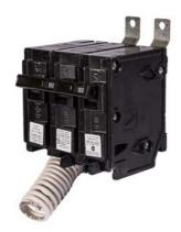
Siemens Low Voltage Molded Case Circuit Breakers Panelboard Mounting 240V Circuit Breakers - Type BL, 2-Pole, 120/240VAC are Circuit Protection Molded Case Circuit Breakers. Type: BL Special Features: Shunt Trip 120V Application: Electrical Distribution Standard: UL 489 Voltage Rating: 120/240V Amperage Rating: 30A Trip Range: Thermal Magnetic Interrupt Rating: 10 AIC Number Of Poles: 2P
