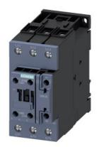
power contactor, AC-3 40 A, 18.5 kW / 400 V 1 NO + 1 NC, 24 V DC with varistor, 3-pole, Size S2, screw terminal Suitable for 2 A PLC outputs
