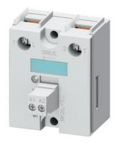
Semiconductor relay, 1-phase 3RF2 Overall width 45 mm, 50 A 48-460 V  $\prime$  4-30 V DC screw terminal
