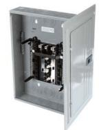
SIEMENS LOW VOLTAGE PL SERIES LOAD CENTER. MAIN LUG WITH 12 1-INCH SPACES ALLOWING MAX 24 CIRCUITS. 3-PHASE 4-WIRE SYSTEM RATED 120/240V OR 120/208V (125A) 100KA INTERRUPT. SPECIAL FEATURES: COPPER BUS, INTERCHANGEABLE MAIN, GRAY TRIM, NEMA TYPE1 ENCLOSURE FOR INDOOR USE.
