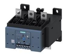
Overload relay 50...200 A for motor protection Size S6, Class 20E Contactor mounting/stand-alone installation Main circuit: busbar connection Auxiliary circuit: Screw terminal Manual-Automatic-Reset
