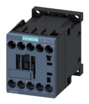
power contactor, AC-3 7 A, 3 kW / 400 V 1 NO, 24 V DC 0.7-1.25\* US, suppressor diode integrated, 3-pole, size S00, screw terminal suitable for PLC outputs not expandable with auxiliary switch
