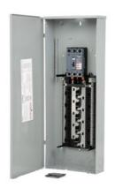
SIEMENS LOW VOLTAGE PL SERIES LOAD CENTER. FACTORY INSTALLED MAIN BREAKER WITH 30 1-INCH SPACES ALLOWING MAX 54 CIRCUITS. 3-PHASE 4-WIRE SYSTEM RATED 120/240V OR 120/208V (200A) 22KA INTERRUPT. SPECIAL FEATURES: COPPER BUS, INTERCHANGEABLE MAIN, GRAY TRIM, NEMA TYPE3R ENCLOSURE FOR OUTDOOR USE.
