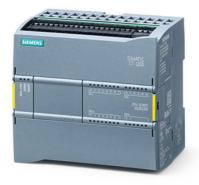
SIMATIC S7-1200F, CPU 1214 FC, compact CPU, DC/DC/DC, onboard I/O: 14 DI 24 V DC; 10 DO 24 V DC; 2 AI 0-10 V DC, Power supply: DC 20.4-28.8V DC, Program/data memory 125 KB
