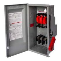
Siemens Low Voltage Circuit Protection Heavy Duty Safety Switches. Type: ENCLOSED, SAFETY SWITCH Std: UL V. Rating: 600V A. Rating: 30 A No. Of Poles: 3P F. Rating: 60Hz Action: SINGLE THROW Material: 304SS Enclosure: TYPE 12. 2-3 point mounting holes. Insulation: YES O. Cycles: 10000 O. Temperature: (-20F-120F) AMBIENT TEMPERATURE Environmental Conditions: INDUSTRIAL
