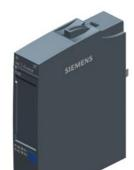
SIPLUS ET 200SP analog input module, Al 4XI 2-/4-wire Standard, -  $40...+70^{\circ}C$  with conformal coating based on 6ES7134-6GD01-0BA1 . suitable for BU type A0, A1, Color code CC03, Module diagnostics, 16 bit, +/-0.3%
