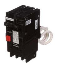
Siemens Low Voltage Residential Circuit Breakers Miniature Circuit Breakers GFCI - Equipment Protect 2-pole plug-on 10k are Circuit Protection Load Center Mains, Feeders, and Miniature Circuit Breakers. Sub Brand: N/A Type: QE Special Features: N/A Application: Electrical Distribution Standard: UL 489 Voltage Rating: 120/240 V Amperage Rating: 20A Load Rating: N/A Frequency Rating: N/A Phase: N/A Frame: N/A Trip Type: N/A Trip Range: Thermal Magnetic Interrupt Rating: 10 AIC Number Of Poles: 2P
