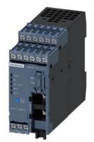
Basic unit SIMOCODE pro V PN, Ethernet/PROFINET IO, PN system redundancy, OPC UA server, Web server, transmission rate 100 Mbps, 2 x bus connection via RJ45, 4I/30 freely parameterizable, Us: 24 V DC, input for thermistor connection Monostable relay outputs, expandable by extension modules
