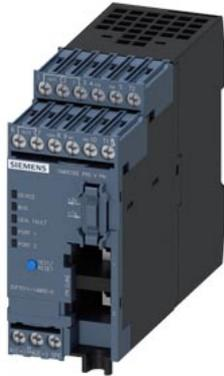
Basic unit SIMOCODE pro V PN, Ethernet/PROFINET IO, PN system redundancy, OPC UA server, Web server, transmission rate 100 Mbps, 2 x bus connection via RJ45, 4I/3O freely parameterizable, Us: 24 V DC, input for thermistor connection Monostable relay outputs, expandable by extension modules
