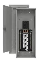
SIEMENS LOW VOLTAGE PL SERIES LOAD CENTER. FACTORY INSTALLED MAIN BREAKER WITH 24 1-INCH SPACES ALLOWING MAX 42 CIRCUITS. 3-PHASE 4-WIRE SYSTEM RATED 120/240V OR 120/208V (150A) 22KA INTERRUPT. SPECIAL FEATURES: COPPER BUS, INTERCHANGEABLE MAIN, GRAY TRIM, NEMA TYPE1 ENCLOSURE FOR INDOOR USE.
