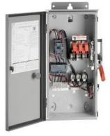
Slim Line Pump Control Panel NEMA size 1 Three phase full voltage Solid-state overload relay OLR amp range 5.5-22A 110/120V 50/60Hz Coil 30A fusible disconnect 30A/600V fuse clip 1NC / 1NO auxiliary contacts HOA Sel. Sw. <(>&<)> Start/Stop 3-point power terminal block 3-point control terminal block 3-point ground lug Enclosure NEMA type 3/3R Weather proof outdoor use
