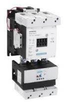
Non-reversing motor starter Size 5 Three phase full voltage Solid-state overload relay OLRelay amp range 55-250A 440-480V 50-60HZ/DC coil Combination type No enclosure
