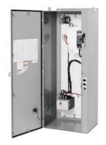
Enclosed soft starter, Controller 3RW44436BC34, Std duty rating 125Hp @460V, Std duty current rating 180A, Control voltage 115 AC, Combination type, 250A circuit breaker, Enclosure type 3/3R, Weather proof outdoor use
