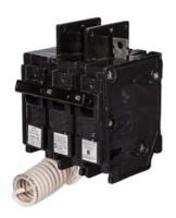
Siemens Low Voltage Molded Case Circuit Breakers General Purpose MCCBs - Type BQ, 2-Pole, 120/240VAC are Circuit Protection Molded Case Circuit Breakers. 2-Pole Common-Trip circuit breaker type BQ. Rated 120/240V (060A) (AIR 10 kA). Special features: 120VAC Shunt Trip. Note: Load side lugs are included.
