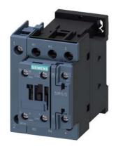
Power contactor, AC-3 25 A, 11 kW / 400 V 2 NO + 2 NC 220 V AC, 50 Hz 240 V, 60 Hz 4-pole Size S0 Screw terminal 1 NO + 1 NC integrated
