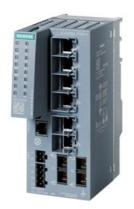
SCALANCE XC206-2 managed Layer 2 IE switch; IEC 62443-4-2 certified; 6x 10/100 Mbps RJ45 ports; 2x 100 Mbps SC ports; 1x console port; diagnostics LED; redundant power supply; temp. range -40 °C to +70 °C; mounting: DIN rail/S7 mounting rail/wall; redundancy functions; Office features (RSTP, VLAN,...); PROFINET IO device Ethernet/IP-compliant C-
