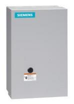
Electrically held lighting contactor, Contactor amp rating 100A, 0 N.C. / 3 N.O. Poles, 110VAC 50HZ/120VAC 60HZ coil, Non-combination type, (no disconnect device), Enclosure NEMA type 1, Indoor general purpose use
