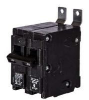
Siemens Low Voltage Molded Case Circuit Breakers Panelboard Mounting 240V Circuit Breakers - Type BL, 2-Pole, 120/240VAC are Circuit Protection Molded Case Circuit Breakers. Type: BL Application: Electrical Distribution Standard: UL 489 Voltage Rating: 120/240V Amperage Rating: 35A Trip Range: Thermal Magnetic Interrupt Rating: 10 AIC Number Of Poles: 2P
